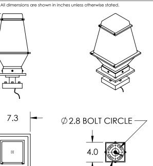
Mounting Method: Mounts Directly To Pier
