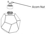
Step 6 (Gem Only): Feed the wiring from LED pendant housing through canopy, followed by the threaded 1/8 IPS. Tighten 1/8 nut down on 1/8 IPS to secure LED pendant housing to Canopy.
